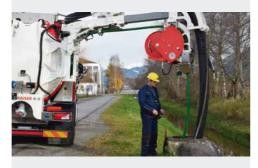
Fast setup due to combined jetting / suction boom; no extensions needed due to vacuum hose reel
