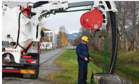
Fast setup due to combined jetting / suction boom; no extensions needed due to vacuum hose reel
