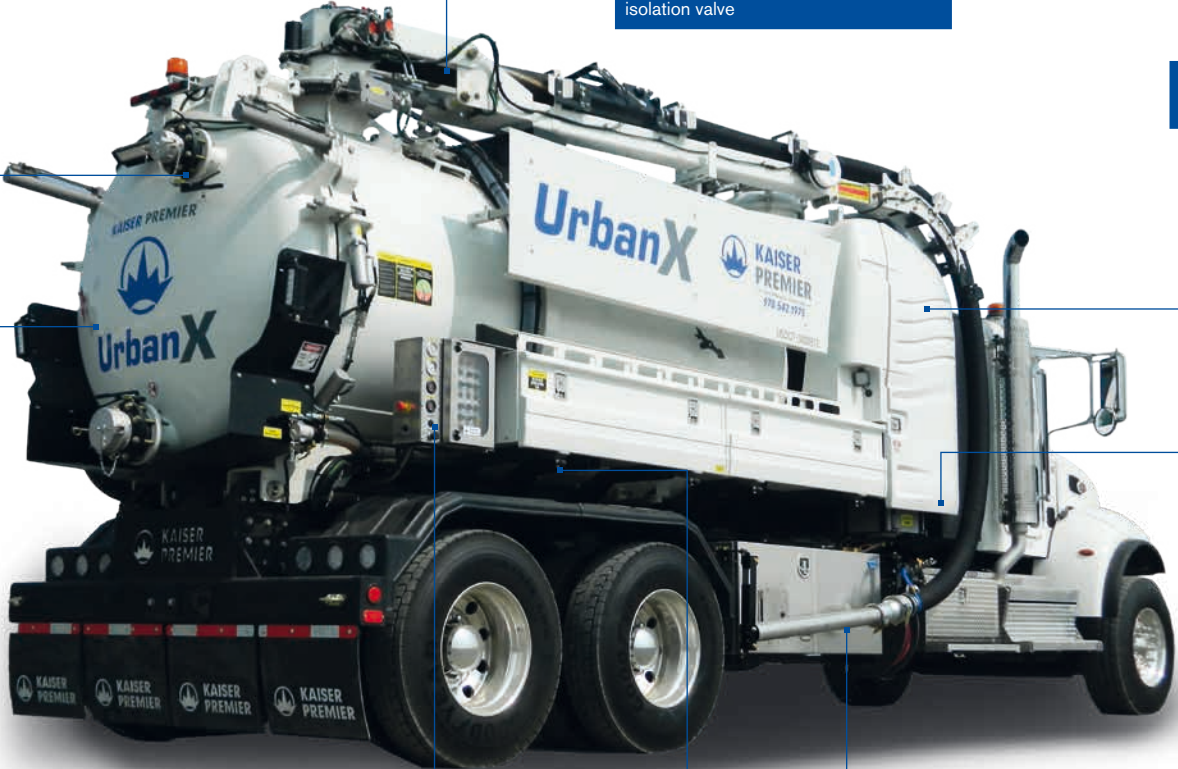
20' Extendable top gun boom with inline isolation valve
