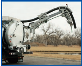
Combined jetting and suction boom for quick and easy setup
